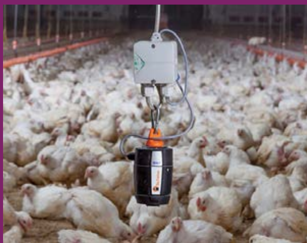
Ammonia meters can be an effective tool to monitor air quality.
